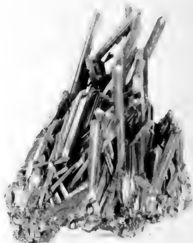
STIBNITE ( to the right ) is a sulphide of the semi-metallic substance known as antimony. The slender orthorhombic prisms are made up of many crystals joined parallel to each other. This mineral is the chief source from which antimony is obtained. The specimen illustrated came from Inyo, Japan
